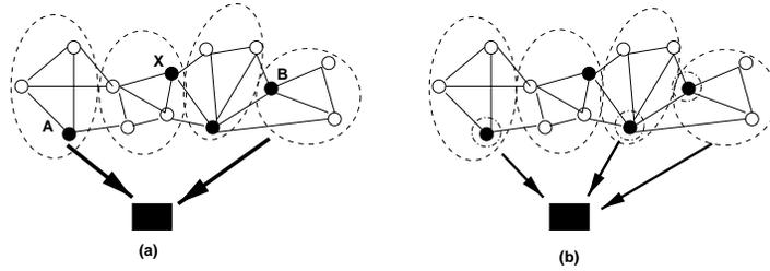
**Figure 1:** *Object Triangulation in Sensor Networks:* The high-level task of this sensor network is to accurately pinpoint the location of the object (represented by a dark square). Under certain assumptions, there exists a localized algorithm which can do this, which may be non-optimal under certain circumstances.
