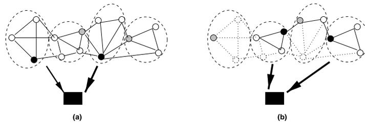
**Figure 2: Adaptive Fidelity Algorithms:** These localized algorithms selectively turn off some sensors to conserve system resources. As individual sensors die, others take their place. This technique extends network lifetime while possibly reducing sensing fidelity.
