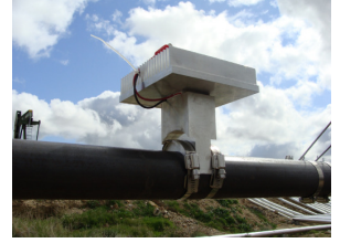
(a) Design of the TEG pipe-mounting apparatus (b) Deployed mount, without extender block
