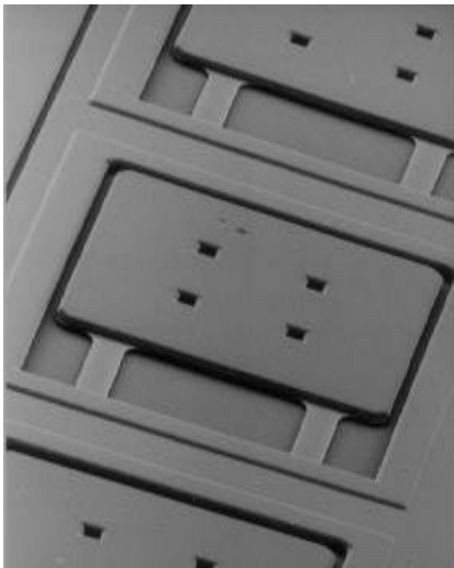
Figure 1: Single cell of permalloy magnetic actuator.
