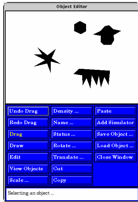
Figure 2: The Object Editor with some sample objects being displayed. The user can define as many objects as desired. Objects are added to the internal database and can be hidden from the user to avoid excessive crowding of the canvas area. Hidden objects have their display status changed to inactive using the function “Status ...”. The function “View Objects” shows all objects defined in the database with their respective display status. The user must use this function to select inactive objects.
