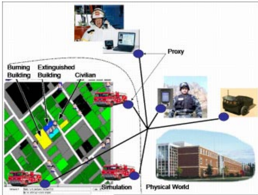
Figure 1: Configuration of experimental platform. Heavy black lines show communication channels between proxies. The dotted line around the bottom left corner shows the division between what is simulated and what is real.
