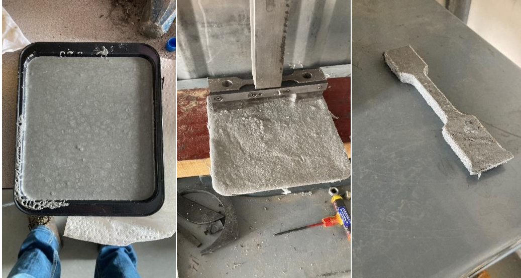
Fig. 1 Cookie cutter tensile specimen manufacturing method.
