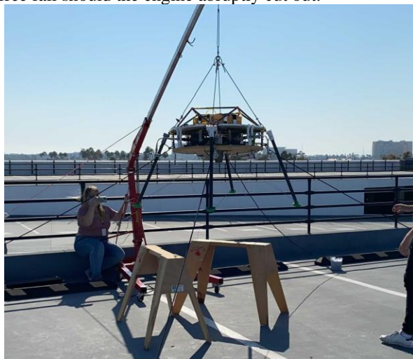
Figure 16: Integrated LEAPFROG supported by the tether test stand
