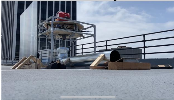
Figure 15: Static hot fire stand prior to test
