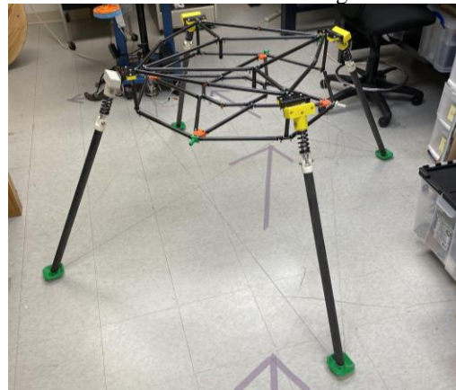
Figure 3: Assembled carbon fiber chassis with legs integrated
