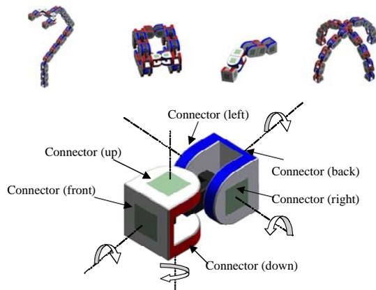
Each Superbot module is a complete robotic system and has a power supply, micro-controllers, sensors, communication, three degrees of freedom, and six connecting faces (front, back, left, right, up and down) to dynamically connect to other modules. This design combines the advantages of many existing reconfigurable robots such as CONRO, PolyBot, MTRAN, and ATRON, and allows flexible bending,
