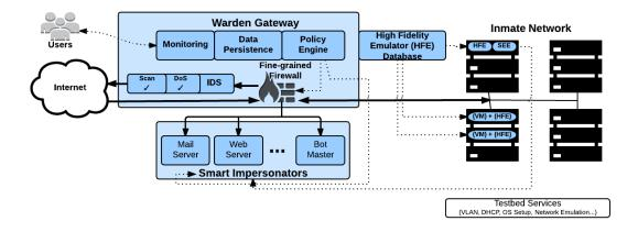
Figure 1: Framework for live malware experimentation on a public testbed.
