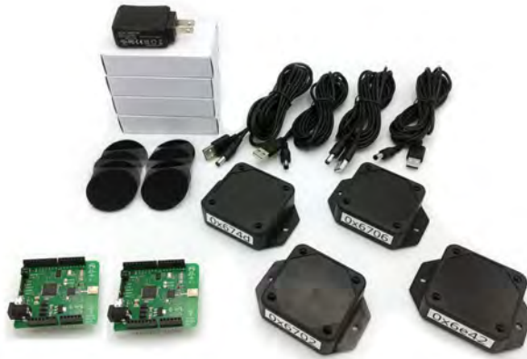
Figure 4.1: The Pozyx multilateration concept. With knowledge of the fixed anchor locations (black squares), the Pozyx tag (green square) will constantly transmit and receive signals to determine its positional state on the testbed (orange).
