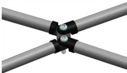
Figure 4: CAD of carbon fibre tube coupling method
