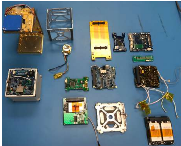
Figure 12: Major satellite bus components prepared before integration
