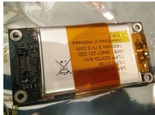
Figure 11: Remote Battery board ready for integration
