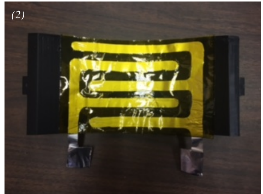
Figure 5: Clamp Geometry (1) (left) and Geometry (2) (right) of electroadhesion samples.
