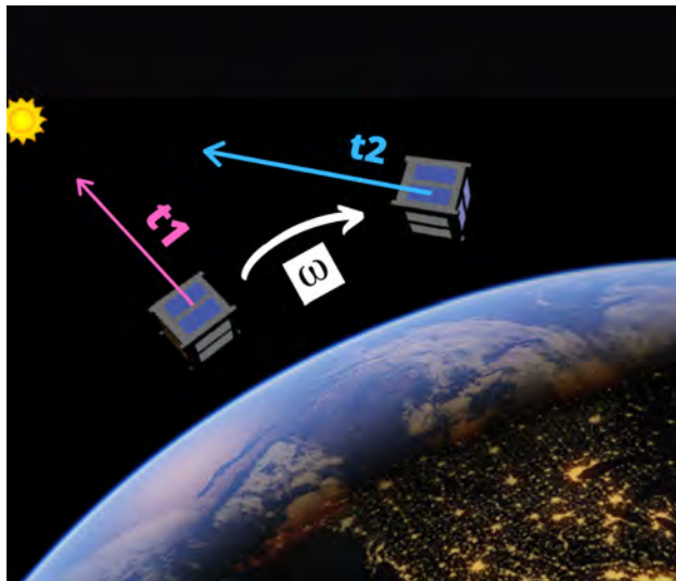
Figure 7: Diagram depicting CubeSat in orbit measuring the sun vector at two different instances, t_1 and t_2 . Gyro readings, \omega , are then used to transform the t_1 measurement into the same frame as t_2 . Once this transformation is completed, the triad algorithm can be followed, taking the sun vector measurement taken at time t_2 to be more accurate and using it to construct the first base vector.
