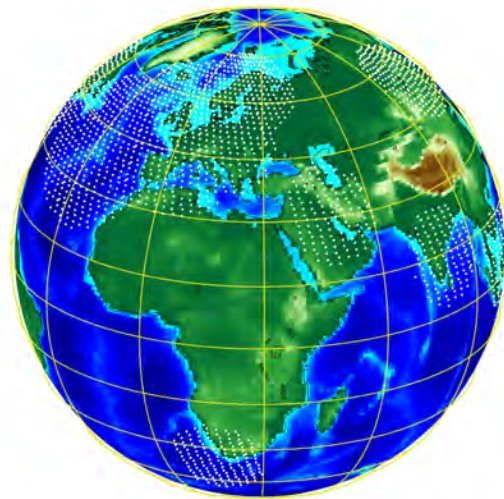
Figure 9: Simulated global coverage of instantaneous magnetometer readings crowd-sourced from amateur ground stations (over a period of 1 month).
