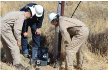
Deployed energy harvesting sensors for cold oil blockage detection research (CiSoft SEN)
