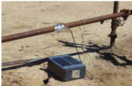
Deployed energy harvesting sensors for cold oil blockage detection research (CiSoft SEN)
