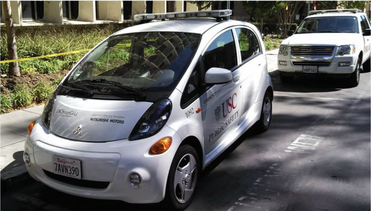
On loan from Mitsubishi, this MiEV vehicle was used for the Smart Grid project. Use data for these electric vehicles was collected by the Smart Grid team for miles driven, type of activity, number of charges and duration of each charge.
