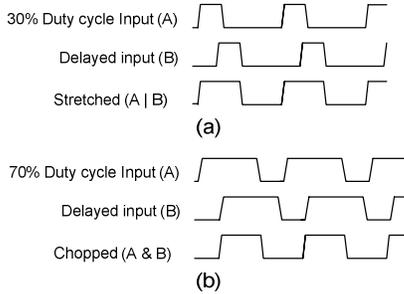
Figure 3. Timing diagram of Stretching and Chopping.
