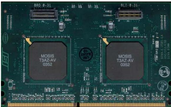
Figure 1. DIVA DIMM with two PIMs.
