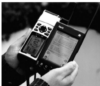
Figure 1: PDA (Palm VII) with GPS device
