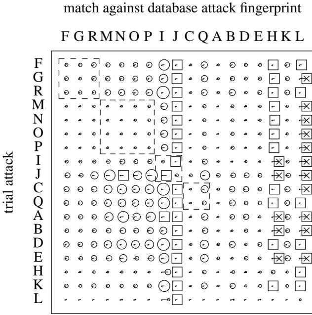
Fig. 4. Graphical representation of  $TA_{XY}$  and  $TP_{XY}$  statistics for 18 attacks captured at Los Nettos (values greater than 1000 is indicated as square and X). Each row represents a trial attack, while each column represents a database fingerprint; the intersection is a comparison of the attack against a particular database entry.
