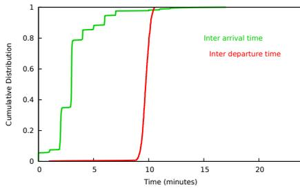
Fig. 8: Comparison of LAX inter-arrival time (for blocks entering E in Figure 1 VS inter-departure time (for blocks exiting E in Figure 1) on one day data.
