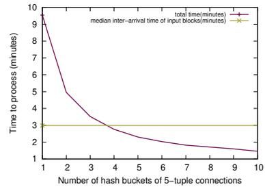
Fig. 9: 4-way connection hashing (on data from A to E in Figure 1) and using 4 Zeek instances on the cluster (as provided by Plumb) is enough to keep up LAX real-time traffic rate.
