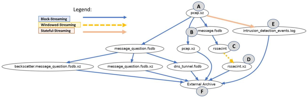
Fig. 1: The DNS processing pipeline, our case study described in §II-A. Intermediate and final data are ovals, computation occurs on each arcs. Different steps use one of our abstractions to achieve diverse processing goals.
