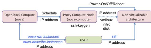
Figure 3. Block diagram of proxy bare-metal compute node
