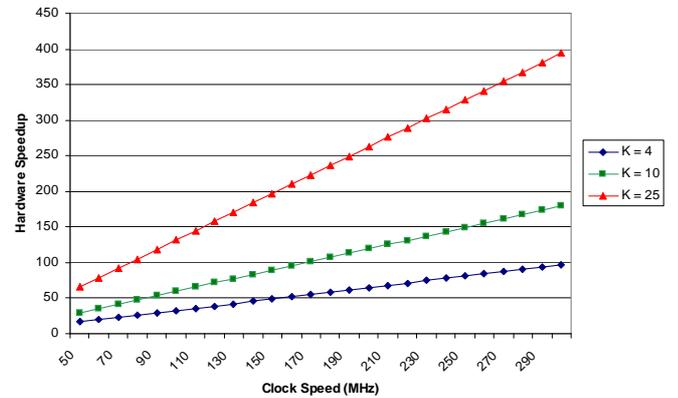
**Fig. 5.** Hardware speedup in comparison to the character implementation in software as clock frequency increases
