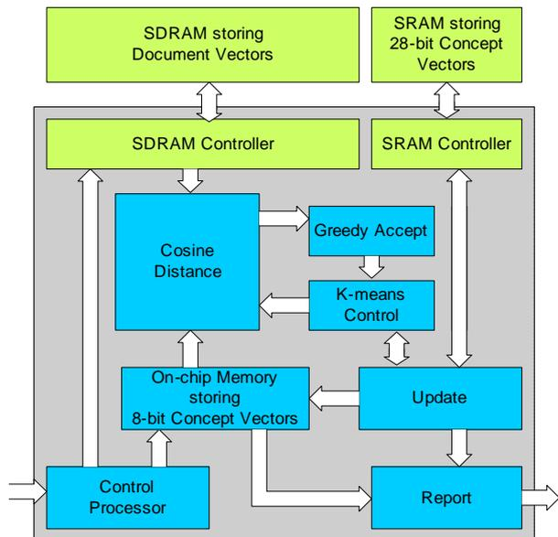
Fig. 3. Hardware Clustering Block Diagram
