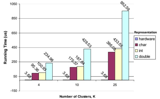
**Fig. 4.** Average time for each software implementation and the hardware implementation comparing one document to all  $K$  concepts.
