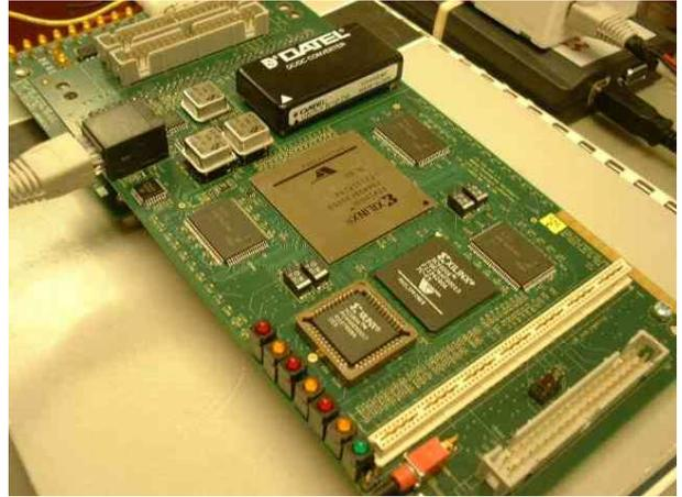
**Fig. 2.** The FPX platform used to implement K-means Clustering
