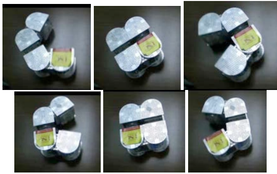
Figure 9: Self-reconfiguration (9a-9f) with SuperBot modules.
